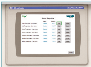
Alarm Setpoints Screen
