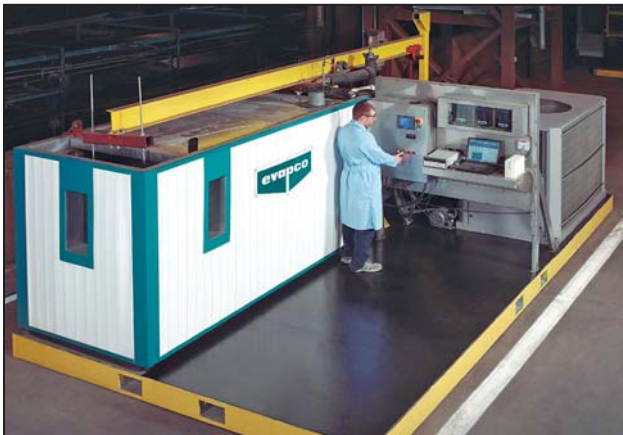
Thermal ice storage test unit with glycol chiller utilized for developing charge and discharge performance ratings
