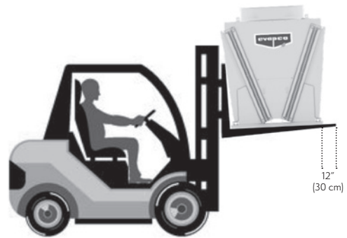
Figure 12 – V-Coil Unit Forklift Lifting Requirements
