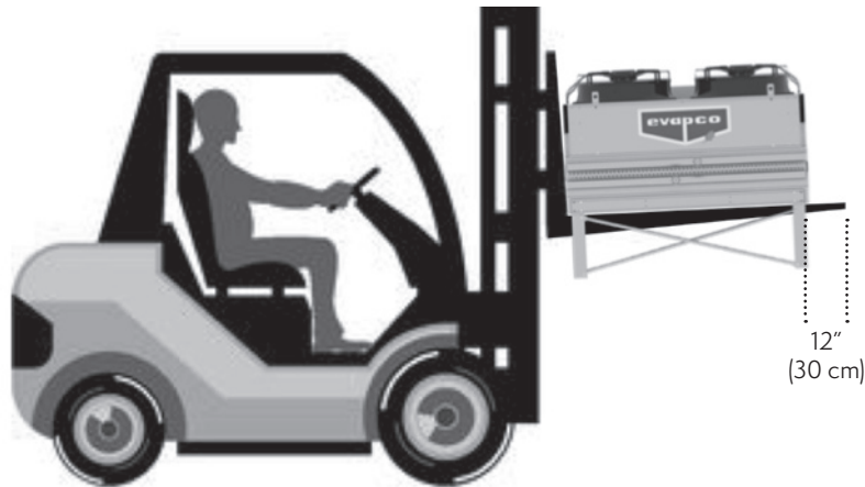
Figure 4 – Flat Coil Unit Forklift Lifting Requirements
